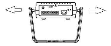
3). There are two washers inside of two holes (the joints of handle and case) respectively. Please use a screwdriver to pry open these washers.
